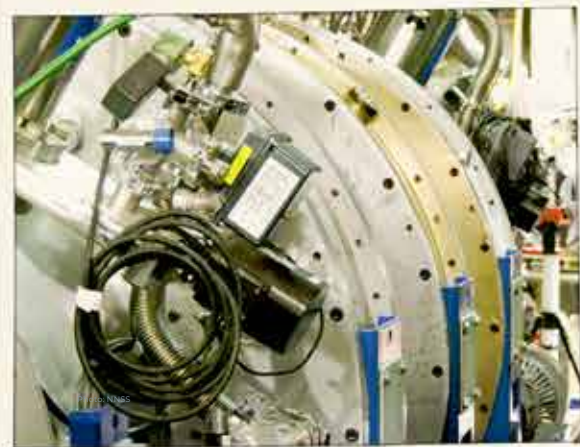
This dual-axis flash x-ray radiography system is used to examine the physical properties of plutonium during subcritical experiments
